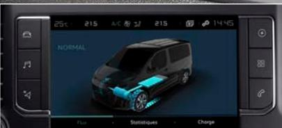
**ENERGY FLOW** : view the operation of the electric technology.
